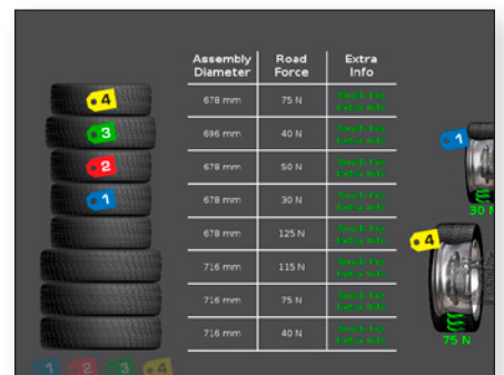
EXCLUSIVE TranzSaver™ Compares tire circumferences as specified by OEs to prevent damage to All Wheel Drive (AWD) vehicles.
